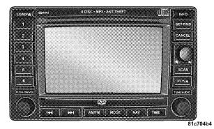
Satellite Navigation Radio with CD Player with MP3 Capability (REC) - combines a Global-Positioning System-based navigation system with an integrated color screen to provide maps, turn identification, selection
